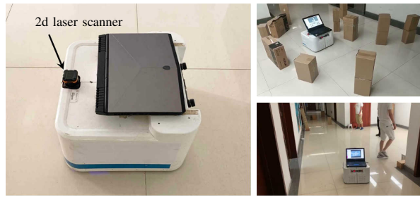
Fig. 7. Our robot chassis with a laptop and a Hokuyo UTM-30LX laser scanner (left). Real test environment(right), including difficult obstacle environments (upper right) and long-range corridor test (bottom right).
